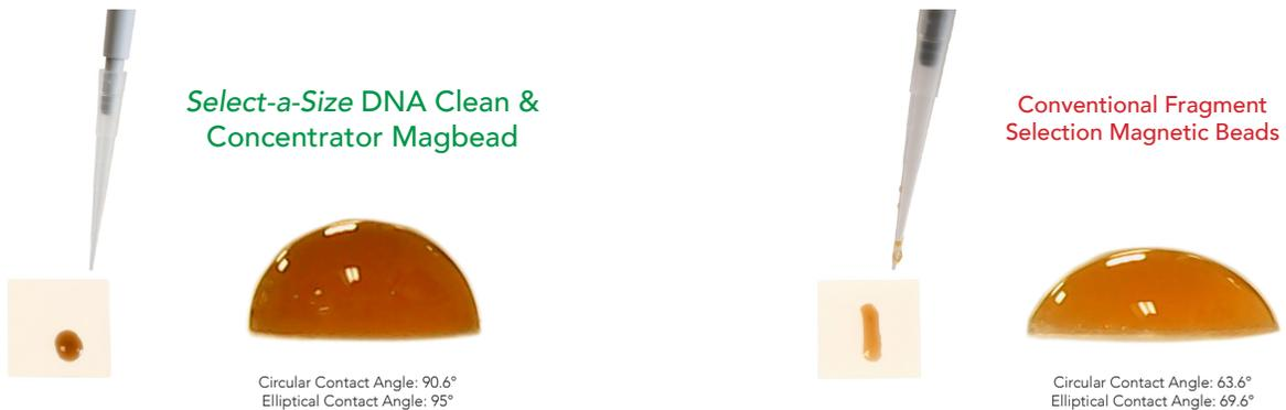
Reduced fluid surface adhesion for improved microliter pipetting. More consistent low volume magnetic bead transfers due to less reagent "stickiness" to pipet tips.
